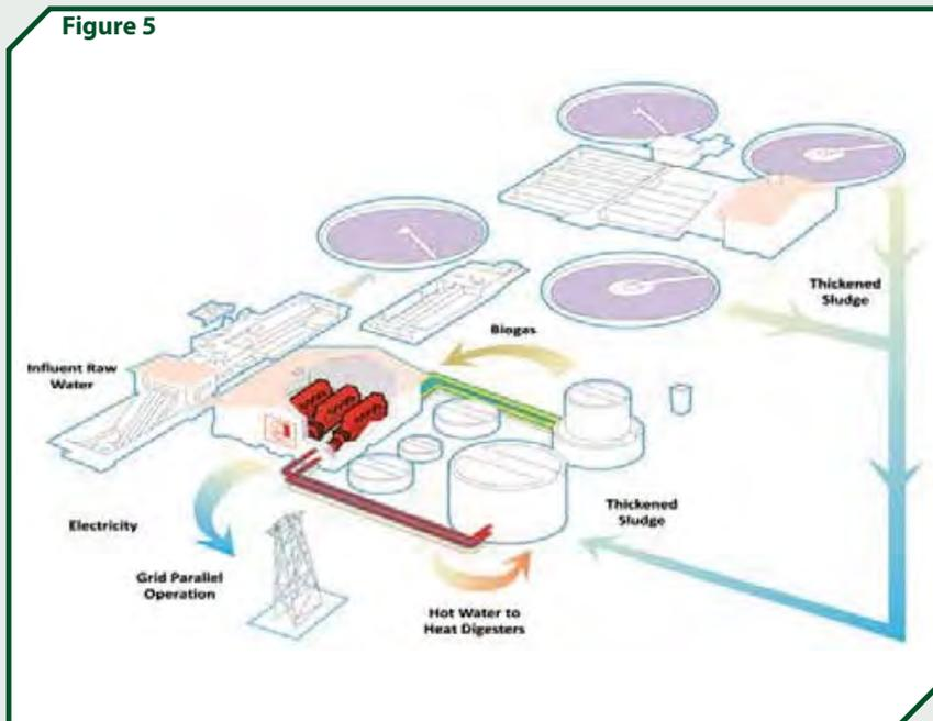
Figure 5: Flow diagram of Waste Water Treatment Works (WWTW) power generation plant: (source: WEC Projects).
