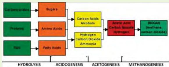
**Figure 1:** Anaerobic digestion process (source: NREL).
